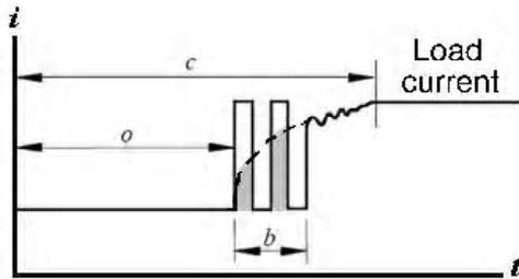
Fig. 6. Oscillogram of relay making process with contact bounce (according to IEC 61810-7): *o* – time period from coil energizing up to first contact closing; *b* – bounce time; *c* – time to stable closing
