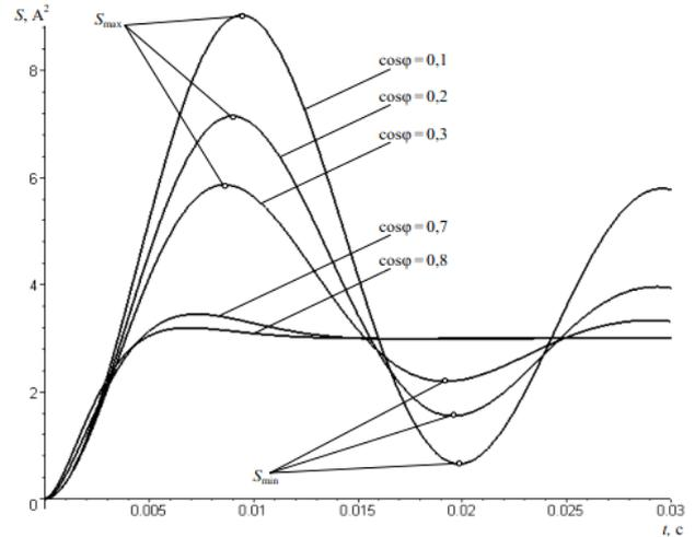
**Figure 3.** The time-current characteristic of selective circuit
