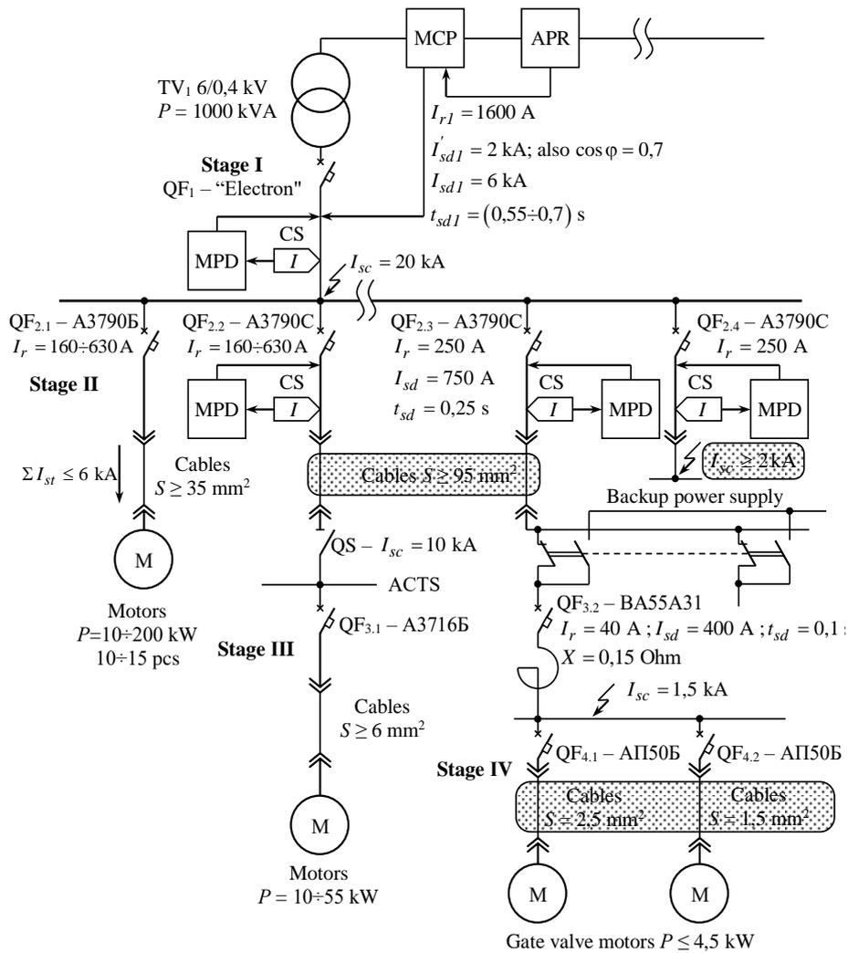
**Figure 1.** Fragment of the generalized diagram of the 0.4 kV auxiliary electrical installation NPP
