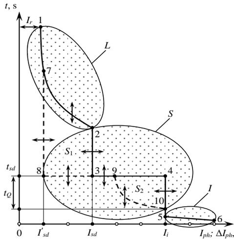
**Figure 4.** Time-current protective characteristic of the breaker operating together with the MPD after modernization:
